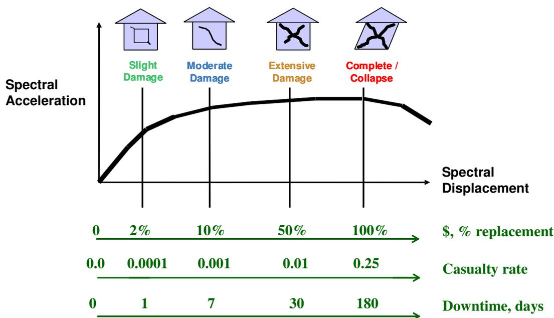
Figure 3 Building loss functions
