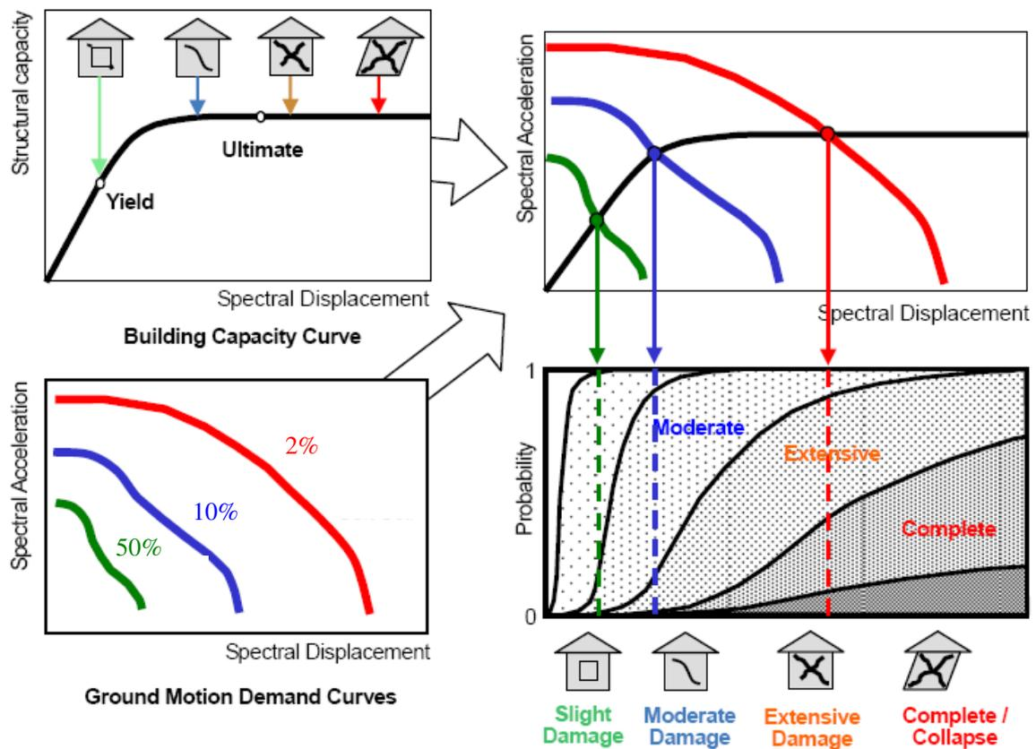
Figure 1 HAZUS earthquake loss estimate methodology for buildings
