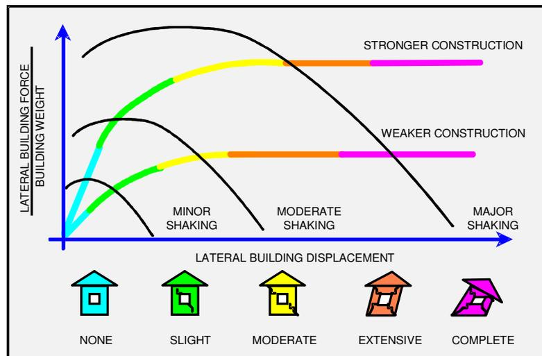
Figure 2 Determination of building response points (performance points) and correspondence between damage states and segments in building capacity curve
