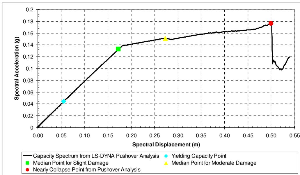
Figure 4 The capacity spectrum and locations of key points
