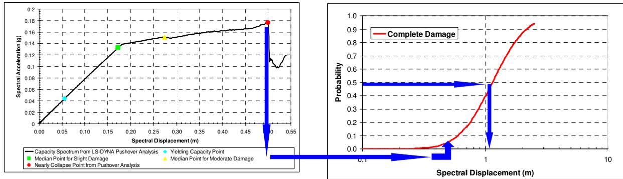
(a) Capacity Spectrum from Pushover Analysis (b) Fragility Curve for the Complete Damage State
