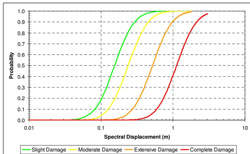
Figure 6 Derived fragility curves for the group of buildings represented by the selected building
