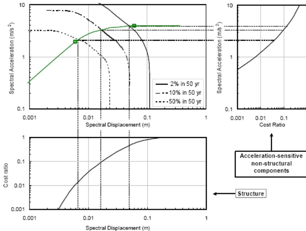
Fig. 15 Damage cost ratios for the structure and non-structural elements of a HAZUS default low-rise unreinforced masonry building subjected to three levels of ground motion
