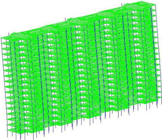
Fig. 11. Deformed shape of a high-rise reinforced concrete moment frame – shear wall (core) building during pushover
