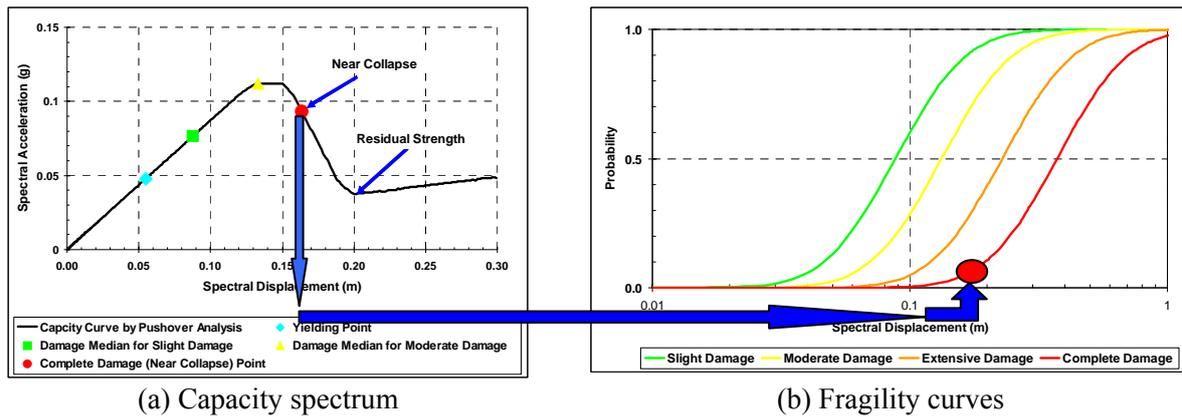
Fig. 13. Determination of the fragility curve for the complete damage state
