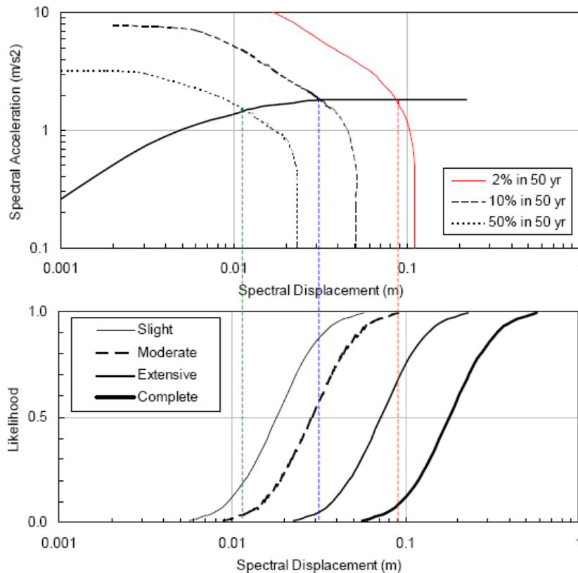
Fig. 6. Example for low-rise concrete frame (CF) buildings using the default HAZUS values for pre-code buildings
