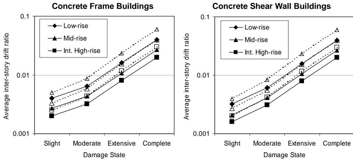
Fig. 16. Default Median Values of HAZUS Fragility Functions for Concrete Buildings; Solid Lines are for Pre-Code Seismic Design and Dashed Lines for Moderate Code Seismic Design
