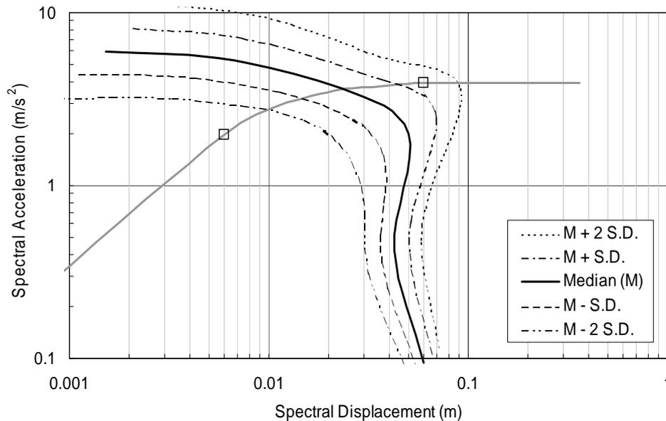
Fig.14. Example for the determination of spectral displacement for a HAZUS default pre-code low rise unreinforced masonry building when subjected to the 2% in 50 year uniform hazard ground motion for site class D shown in Figure 2
