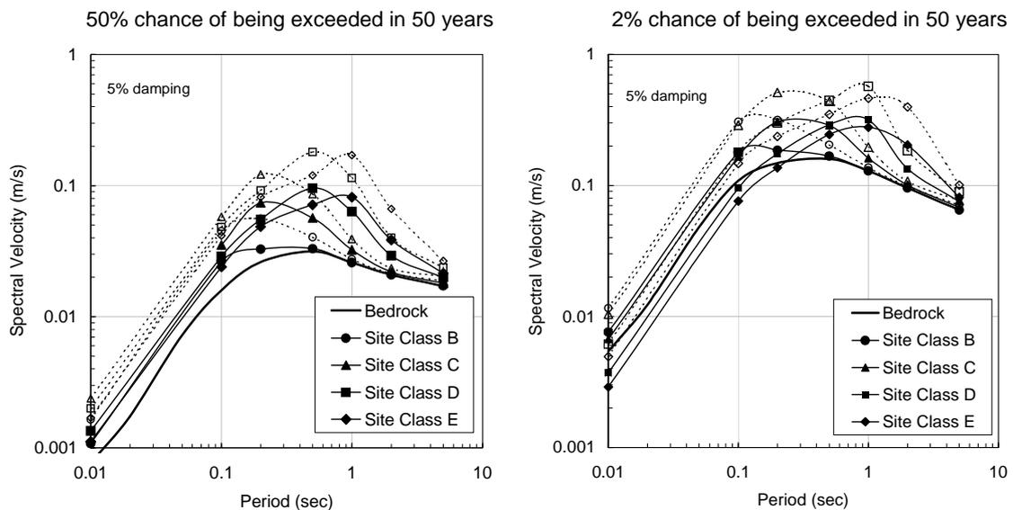
Fig. 2. Horizontal velocity uniform hazard response spectra for various Site Classes (Pappin et al., 2004)
