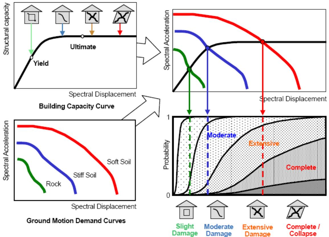
Fig. 3. HAZUS earthquake loss estimate methodology for buildings
