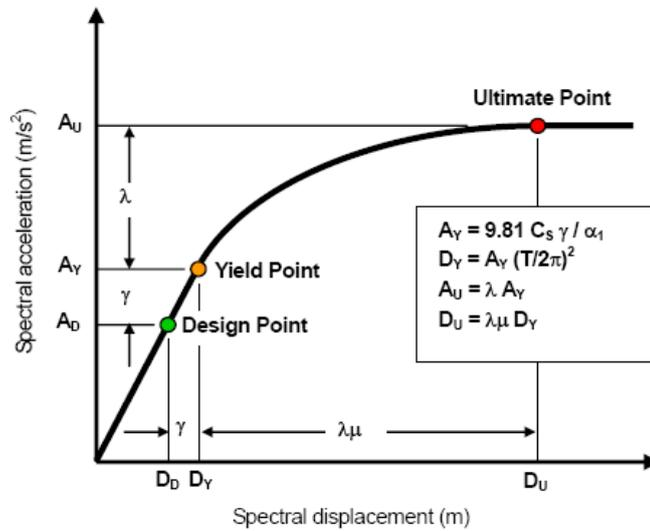
Fig. 4. HAZUS capacity curve definition
