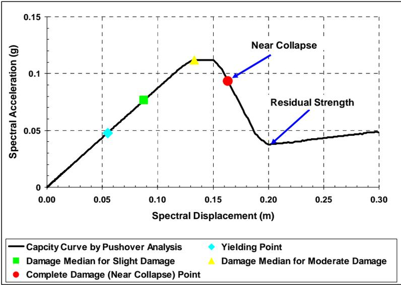
Fig. 12. The capacity spectrum from the nonlinear pushover analysis
