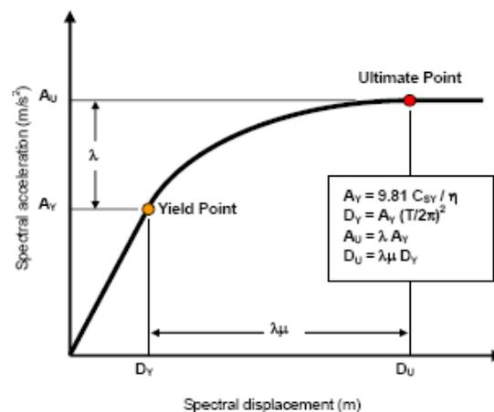
Fig. 7. Definition of capacity curve
