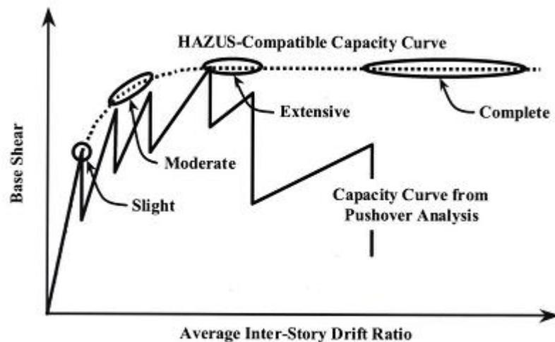
Fig. 10. Example damage state medians from “Saw tooth” Pushover curve, FEMA (2000)
