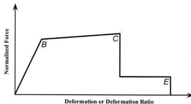
Fig. 9. Idealized force deformation curve, FEMA (2000)
