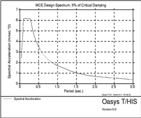
**Figure 2:** Design earthquake response spectrum
