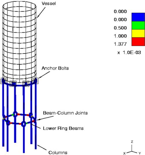
Figure 4: Maximum plastic hinge rotation angle of the retrofitted structure
